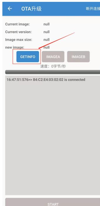
4. Download the product upgrade firmware and move it to the designated storage directory under the mobile phone's file system. If the current hardware information is imageB, place the upgrade firmware in the "internal storage device\CH5730TA\imageA" directory. If the current hardware information is imageA, place the upgrade firmware in the "internal storage device\CH5730TA\imageB" directory.
