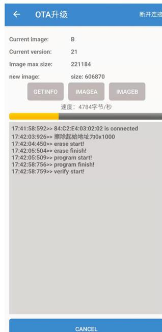
8. Wait for the upgrade process to complete. After the end, wait for the Bluetooth device to disconnect or click "Disconnect" in the upper right corner to actively disconnect the connection.
