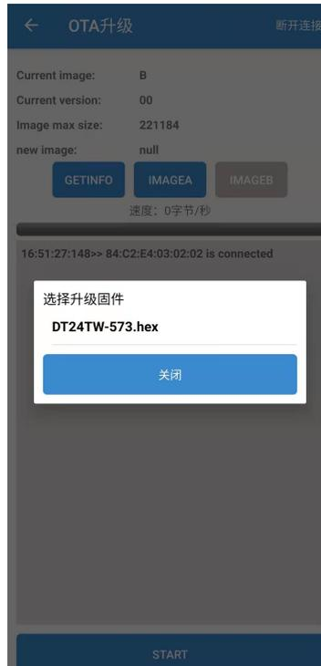
6. After selecting the file, click the "START" button below to start the upgrade. If the selected upgrade file is a HEX file, the APP will automatically obtain the address where it is erased. If the selected upgrade file is a BIN file, the user needs to manually specify the starting address for erasure.
