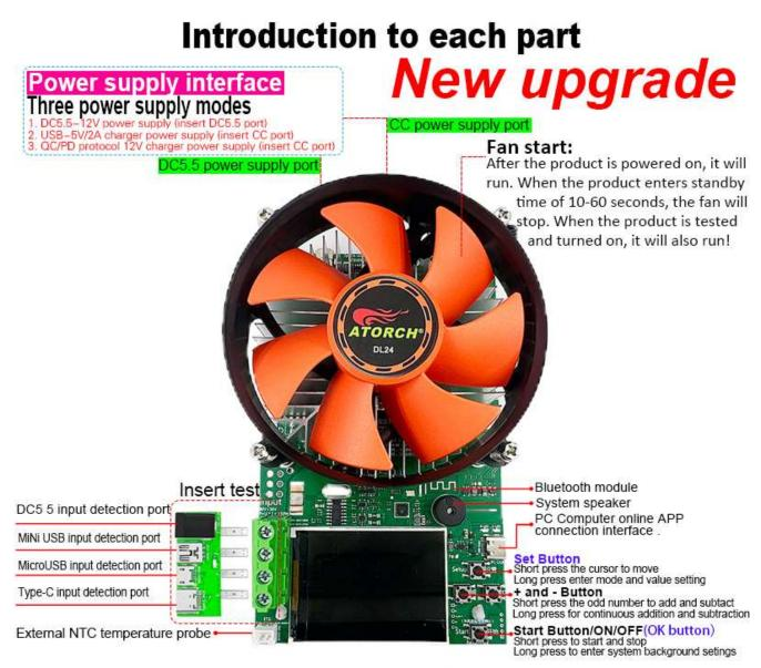
Data reset zero operation button: Press and hold the Set button and OK button at the same time to reset capacity(mah) and energy data(Wh)!
