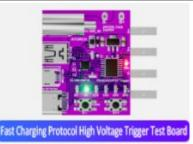
Load Fast Charging Protocol High Voltage Trigger Test Board This load test board can support PD3.1 compatible with PD3.0 protocol, QC, AFC, FCP and other protocols. By sending fast charging protocol chargers or power banks, it can triggered 5V/9V/12V/15V/20V/28V fast charging voltage for various aging and testing, as well as quality identification, voltage, current and power identification.
