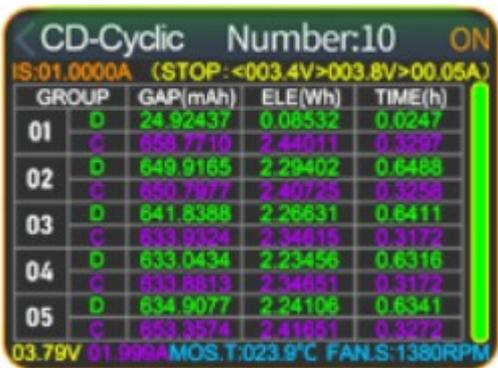
Select the CDxN charge and discharge cycle test function on the menu interface, press briefly to enter this function follow the wiring diagram as shown in the figure, and then press the start button. The entire process will automatically cycle and detect 1-99 group sets of values The discharge aging detection performance is simple and convenient.
