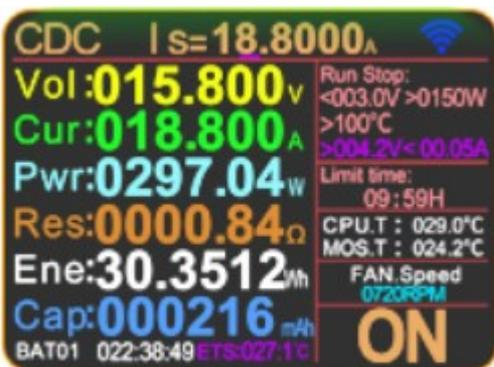
When selecting the CDC function on the menu interface , simply follow the wiring instructions in the following diagram, Press the“OK/Start”button again to perform a fully automatic charge and discharge . (CDC) cycle test.
