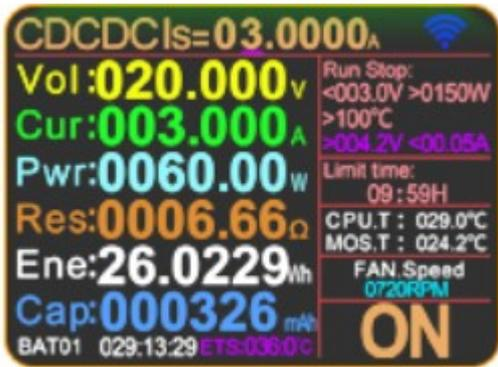
When selecting the CDCDC function on the menu interface simply follow the wiring instructions in the following diagram, Press the “OK/Start” button again to perform a fully automatic charge and discharge . (CDCDC) cycle test.
