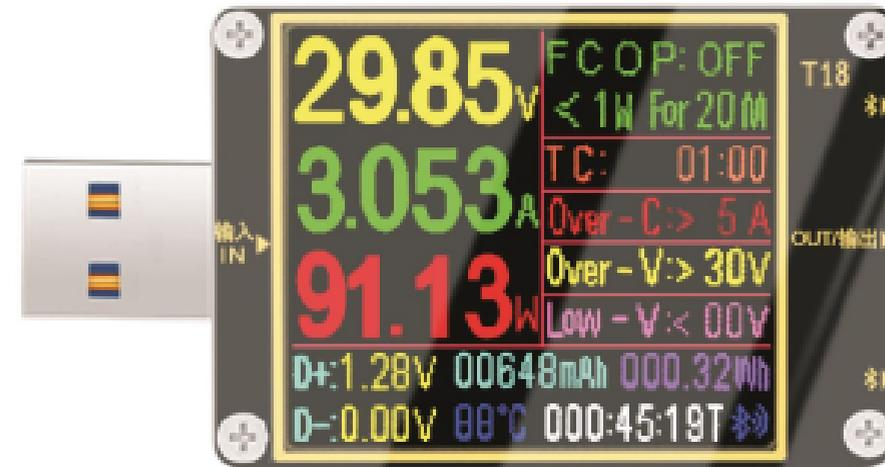
Universal detection of various USB devices, a variety of DC power supply, a variety of battery capacity parameters and power-off protection during charging.
