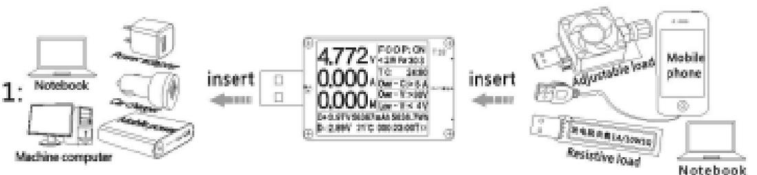
Variety USB&DC Power USB&DC Detector (main interface) Various electronic load or other equipment
