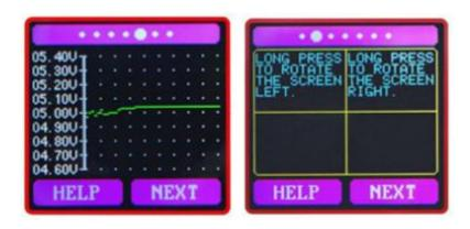
This interface is voltage measurement waveform diagram. It automatically changes the range within the range of 4.5-24V measurement and displays voltage fluctuations in real time.
