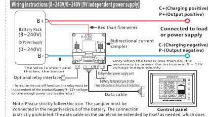
not affect the data transmission and measurement accuracy.  ${f 1}$  ) The sampler of this Meter must be connected to the negative electrode circuit of the battery pack. The B-
