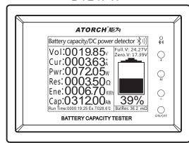
This user manual is applicable to 100A/200A/300A/400/500A/600A/1000A This equipment is used to measure and display the voltage, current, power, analog load resistance value, discharge capacity, electricity quantity, battery temperature, over-voltage prompt, low-voltage prompt, over-power prompt of the battery pack/power supply, as well as the percentage value of electricity quantity corresponding to the battery voltage ratio
