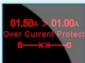
Overcurrent automatic power off alarm interface
